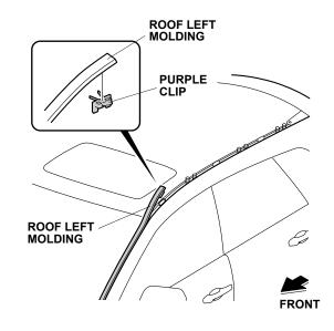
15. Reinstall the roof left molding cover.
