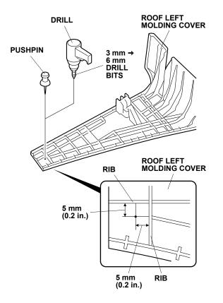
4. While wearing eye protection, drill the pierced mark with a 3 mm drill bit. Enlarge the hole with a 6 mm drill bit. Remove any burrs.
