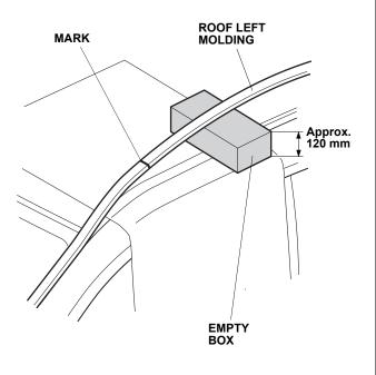
9. While wearing eye protection, use an air saw to cut the roof left molding at the mark. Do not use a cutting wheel or shears tocut the molding, it will damage the roof left molding. Have an assistant hold the rear edge while cutting.
