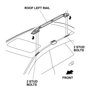
27. Secure the roof left rail to the left center stay with two short Torx bolts. Torque the short Torx bolts to  $7-12 \text{ N} \cdot \text{m}$  (5-9 lbf-ft).
