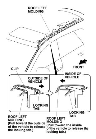
7. Place a blanket over the roof of the vehicle under the mark on the roof left molding. Be careful not to deform the roof left molding when measuring and cutting.
