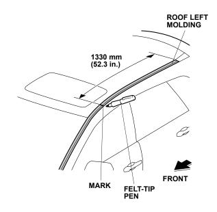
6. Pull the roof left molding toward the outside of vehicle to release the locking tab, press the locking tab toward the inside of vehicle, then release the roof left molding from the vehicle. When removing the roof left molding, start from the rear of the vehicle and work towards the front.
